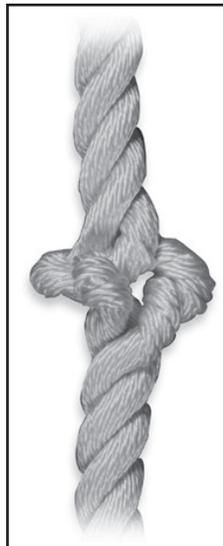
If, on the other hand, the line is continuously hauled over a winch in a clockwise direction, the rope lay is shortened and the rope becomes stiff and will kink readily.
