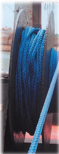
2. On the storage half of the split drum winch, the first two or three layers of AmSteel-Blue should be reeled on under some tension to create a solid, smooth base layer. After these layers, the rope on the storage side can be laid on in layers with some crossovers. These crossovers should prevent the AmSteel-Blue from diving in-between the layers and getting stuck during deployment.
