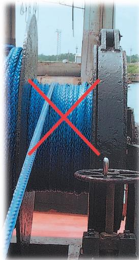
**LEFT:** Line installed incorrectly on working side of winch drum! On working side of winch, only wrap a single layer of line (8 wraps). Working part of line should come off end of wraps, not from the middle as shown above.
