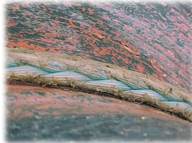
*Line installed on storage side of winch drum. Cross-overs prevent AmSteel-Blue from diving between layers and getting stuck during deployment.*
