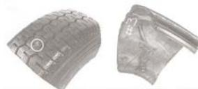
Driving the tire a short distance while it was severely under-inflated caused this dangerous, non-repairable condition shown above. The damage was not visible from the outside. Every tire must be removed from the wheel for inspection and to assess reparability.
