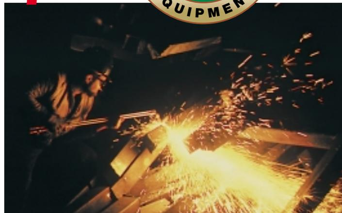
*Reverse flow can occur as a result of a blocked torch tip, excess gas or oxygen pressure, lack of pressure, or unsafe start-up or shut-down procedures.*
