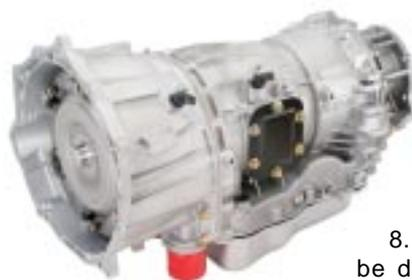
Another transmission that uses the 29 spline output shaft and fits up to the Atlas is the ZF manual 6 speed (ZF S6-650). This transmission is a 29 spline when coupled to the Duramax and the 8.1L. The Allison 4WD 5 and 6 speed automatic is also a 29 spline transmission when coupled to the same Duramax and the 8.1L. These transmissions can be directly mounted to the Atlas transfer case. The Atlas must be equipped with a special case rotation for these applications.
