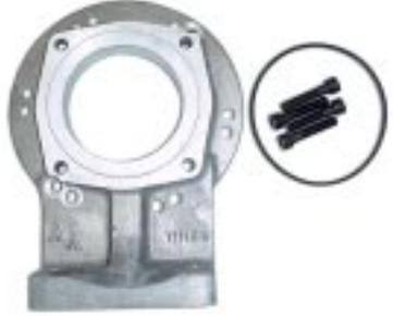
**P/N AS-6401** - Includes a 1.25" adapter, a gasket, and 6 standard socket head cap screws.
