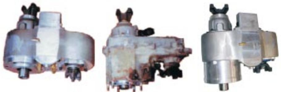
The Atlas 2 speed (left) & Atlas 4 speed (far right) in comparison to the NP231 (center) with a fixed yoke kit
