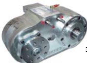
We also offer a kit to retrofit an Atlas from a 26 spline to a 32 spline front output. This upgrade kit can also be installed into any previously built Atlas. Instructions are provided online for mechanically inclined individuals to perform this upgrade.
