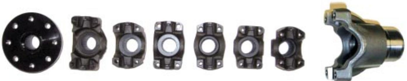
**Yoke Modifications:** Changing the style of yokes on the Atlas transfer case may require your new yoke to be modified. When installed on an Atlas, the yoke will load up against a tapered roller bearing. Some yokes require a chamfer to be machined to clear the cage of this bearing. The yoke drawing shows the required machining on these yokes.
