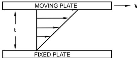
Mathematically, the absolute viscosity is defined as the ratio of shear stress to shear rate, or
