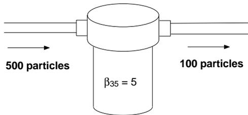
Example: A filter with " $\beta_{35} = 5$ " means for every five particles greater than or equal to 35 $\mu$ m encountering the filter, one of those particles passes through the filter. This filter has a filter efficiency of  $E_{35} = 100(1 - 1/5) = 80\%$ .
