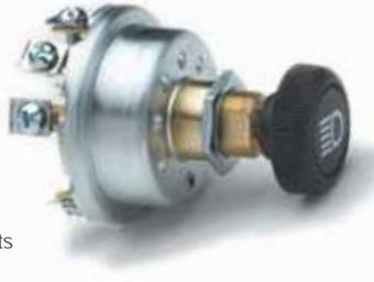
With black knob imprinted with SAE headlamp symbol. Silver contacts. Five screw terminals. Plated steel case. Mounting stem 5/8"-32 thread. With O-ring seal in the mounting stem. 20A per circuit at 12V DC.
