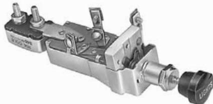
Rotation of knob dims panel lights in Mid and Out knob positions. 3.75 Ohm Dimmer, 30A at 12V Circuit Breaker. With black knob imprinted 'Lights'. Four screw terminals. Plated steel case. Mounting stem 3/8"-24 thread.
