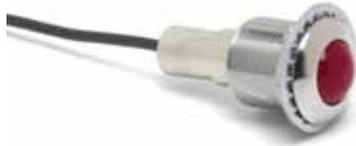
12V #53 bulb supplied. 17/32" (14.5mm) diameter lens. 3/4" (19.1mm) diameter mounting stem, 11/16" (17.5mm) long. Chrome-plated brass bezel, 7/8" (22.2mm) diameter. Available with custom imprinting: contact Cole Hersee.
