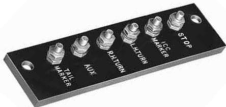
Six-gang, with circuit identification printed in white lettering. Two mounting holes 5.25" (133.4mm) on centers. 10-24 thread stud terminals, with hexnuts. 4 7/8"L x 1 3/16"W x 3/4"H (149.2 x 38.1 x 19.1mm).
