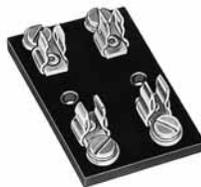
For SAG (AGU) fuses 13/32" diameter x 1 1/2" long (10.3 x 38.1mm), rated up to 60A. Screw terminals, phosphor-bronze fuse clips. Molded plastic base with two 3/16" (4.8mm) mounting holes, .812" (20.6mm) on centers.
