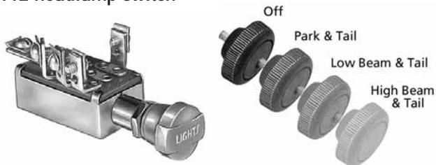
Five screw terminals. Plated steel case. Mounting stem 3/8"-24 thread. With tan knob imprinted 'Lights'. 10A at 12V DC.
