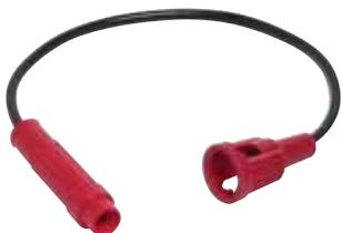
Accepts SFE fuses through 20A and 3AG (AGC) fuses through 30A. Positive twist-lock seal will not open accidentally; large brass contacts maintain solid contact with the fuse for maximum efficiency. 14AWG wire leads, 8" (203.2mm) long. Brass contacts. To install, cut wire loop.
