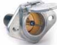
Self-grounding. Solid brass 3/8" (9.5mm) diameter male contact, with insulated tip to prevent short circuits. Rubber boot protects the terminals and connections from moisture and dirt. Fits 2" (50.8mm) diameter hole. Two mounting holes on the flange 21/64" (8.6mm) diameter, 2 5/16" (74.6mm) on centers.
