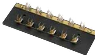
6-gang. Blade terminals on one side of the fuse clip. 5 3/4"L x 1 7/8"W x 23/32"H (146.6 x 47.6 x 18.3mm). Brass terminal screws with lockwashers. Solid brass busbar. Two mounting holes 11/16" (4.3mm) diameter, 3.75" (95.3mm) on centers.
