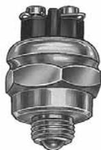
35A at 12V DC. Silver contacts. Transmission-mounted, extra heavy-duty. Compact design for mounting in areas where space is limited. Two female bullet terminals. 9/16" -18 thread mounting stem, 5/16" (7.9mm) long. Replaces: Chrysler 1343998, 2198779, Motorcraft SW-410
