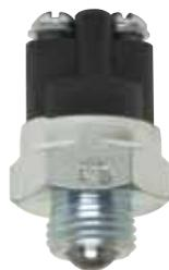
20A at 12V DC. Silver contacts. Transmission-mounted, extra heavy-duty. Compact design for mounting in areas where space is limited. Two screw terminals. 9/16" -18 thread mounting stem, 5/16" (7.9mm) long. Replaces: Autocar 8E-01360, Brockway 128537, Diamond Reo 560-65, Kenworth AT-91-69 Mack 1MR-1320, Oshkosh 13320-F1, White 1743529.
