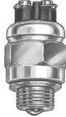
Two female bullet terminals. Mounting stem 3/4" -16 UNF-2A thread, 31/64" (12.3mm) long, with aluminum gasket/washer.
