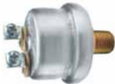
Mounting stem: 1/4" -18 dryseal thread 15/32" long. Insulated. Normally closed, open at 55 - 65 psi (379.2 - 448.2 kPa). 8-32 screw terminal.
