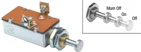
Normally On. Pull-out feature permits circuit to be shut off manually when the door must remain open and operation is not required. 7/16" -20 thread mounting stem, 7/16" (11.1mm) long. Two flats on stem for mounting in double-D hole. Two screw terminals. Plunger is 7/32" (5.6mm) long at On, 3/4" (19.0mm) at Off. 10A at 12V DC.
