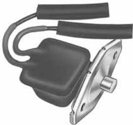
15A at 12V DC. With special diaphragm/mounting bracket, sealed to protect the mounting shaft. Plasticized body protects against moisture and dirt. Two 16AWG wire leads, 3" (76.2mm) long with female bullet terminals. Insulator sleeves protect the connections. 13/64" (5.2mm) diameter mounting holes, 1 1/2" (38.1mm) on centers. 1/4" (6.4mm) long plunger.
