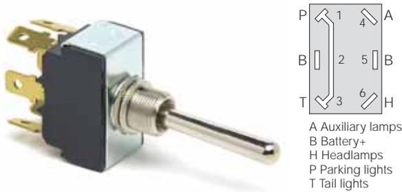
Up: Park, Tail & Headlamps - Center: Off - Down: Park, Tail & Auxiliary Lamps. Six blade terminals. Long handle.
