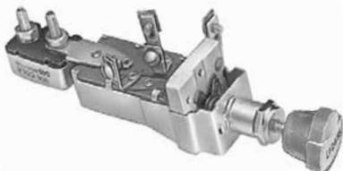
Rotation of knob dims panel lights in Mid and Out knob positions. 11 Ohm Dimmer, 20A at 12V Circuit Breaker. With tan knob imprinted 'Lights'. Four screw terminals. Plated steel case. Mounting stem 3/8"-24 thread.
