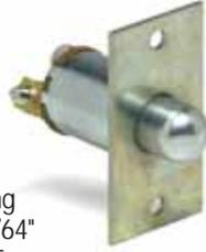
Two 9/64" (3.57mm) diameter mounting holes, 1 3/8" (34.9mm) on centers. 45/64" (17.9mm) diameter plated steel case. Two screw terminals. Plunger: 7/16" long (11.1mm). 5A at 12V DC.
