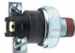
Contacts close at 2 - 5 psi (13.8 - 34.5 kPa). 8-32 screw terminals. Insulated.
