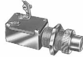
10V at 12V DC. Chrome-plated button. One screw terminal with lockwasher. 5/8"-32 thread mounting stem, 7/8" long (22.2mm).
