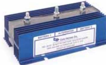
Same as 48160, but with Schottky diodes. Terminations: three 5/16" (7.9mm) studs. Four 9/32" (7.2mm) diameter mounting holes. Size: 8 1/2"L x 4 3/16"W x 3 13/32"H (215.0 x 122.2 x 86.5mm).
