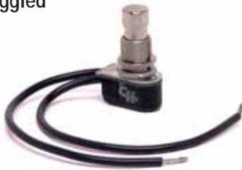
10A at 12V, 5A at 24V. Two 6" (152.4mm) wire leads, 16AWG (1.00mm<sup>2</sup>). Phenolic body, 1.080"L x .530"W x 1.10"H (27.4 x 13.5 x 28.0mm). Push-button diameter .410" (10.4mm). Stem: .470" long (11.9mm). Can be used as a foot switch in dry environments.
