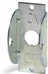
Guard is easily added to an already installed switch, providing lateral mechanical protection. For switches with 15/32" diameter mounting stems with a keyway. Stamped On, Off. 1" x 2.125" (25.4 x 54.0mm). Two .140" (3.6mm) mounting holes 1.87" (47.6mm) on centers.
