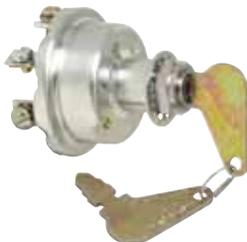
Electrical ratings at 12V DC: 70A Start, 1A Magneto. Three screw terminals. Plated steel case. 5/8" -32 mounting stem with O-ring seal, fits panels up to 1/4" (6.4mm). Long Hencol key.
