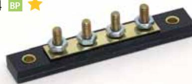
4-gang, with solid brass busbar. 10-32 stud terminals with hexnuts and lockwashers. Two eyelets for mounting with 3/16" (4.76mm) screws (not included). Eyelets are 3.125" (79.4mm) on centers. Moisture-repellent thermoset plastic insulator base. 3 7/8"L x 5/8"W x 27/32"H (44.4 x 15.9 x 21.4mm).
