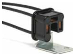
Accepts standard 3-prong flasher units (not included). Molded plastic connector has 14AWG wire leads, with phosphor-bronze contacts. Comes with plated steel bracket that has two .203" (5.2mm) diameter mounting holes.
