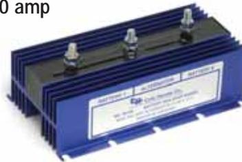
Terminations: three 5/16" (7.9mm) studs. Four 9/32" (7.2mm) diameter mounting holes. Size: 8 1/2"L x 4 3/16"W x 3 13/32"H (215.0 x 122.2 x 86.5mm).
