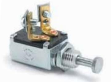
7/16" -20 thread mounting stem, 7/16" long (11.1mm), two flats on stem for mounting in double-D hole. Two screw terminals, plated steel case. 10A at 12V DC.
