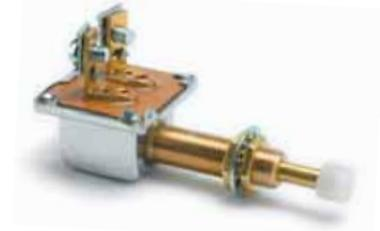
Two brass screw terminals. Brass mounting stem 3/8"-32 thread, 1" (25.4mm) long. Fits panels up to 3/4" (19.1mm) thick.
