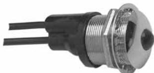
Red lens. Chrome-plated brass bezel, 7/8" (22.2mm) diameter. 3/4" (19.1mm) diameter mounting stem, 11/16" (17.5mm) long, 3/4-32 UN-2A. 5/16" (7.9mm) diameter lens. 12V #56 bulb supplied.
