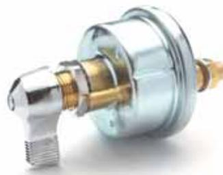
Diecast lever. Plated steel case. Silver-laminated contacts. Brass mounting stem 3/4" -16 thread 17/32" (13.5mm) long. Fits panels through 1/4" (6.4mm) thick. Two 3/8" -24 and two 10-32 studs. O-ring seal in the operating shaft, and gasket-sealed terminal insulator.
