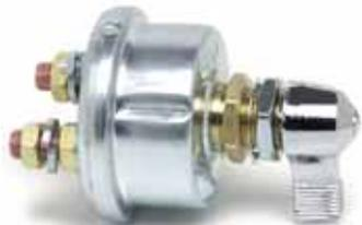
Chrome-plated diecast lever. Plated steel case. Brass mounting stem 3/4" -16 thread 23/32" (18.3mm) long. Fits panels through 3/16" (4.8mm) thick. Two 3/8" -24 and two 10-32 studs.
