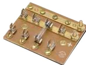
For SFE 20A or 3AG (AGC) fuses. Common hot feed to four independently-fused circuits, and common ground strip for four circuits. Solid brass busbars, terminals and terminal screws. Nickel-plated phosphor-bronze fuse clips. Two eyelet holes for mounting with 3/16" (4.8mm) screws, 2.25" (57.2mm) on centers. 3 1/2"L x 2 3/4"W x 25/32"H (88.2 x 69.8 x 19.8mm).
