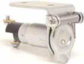
Plated steel housing. High impact-resistant molded plastic insulator. Brass contacts and brass screw terminals. Stainless steel spring on the cover locks the plug in place. Integral mounting bracket with two .218" (5.6mm) diameter mounting holes, 1.25" (31.8mm) on centers.
