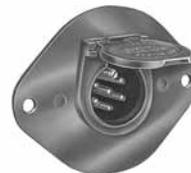
Mounting holes on the flanges : 5/16" (7.9mm) diameter, 4 1/2" (114.3mm) on centers, with additional knockouts 2 15/16" (74.7mm) on centers. Mounts through 2 5/8" (58.7mm) through 3 7/8" (98.4mm) diameter hole.
