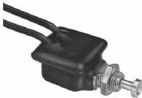
PVC-coated body for moisture and dirt protection. Two 7" (177.8mm) wire leads. Mounting stem: 7/16"-20 thread, .44" (11.2mm) long. Steel button, .38" (9.7mm) diameter.
