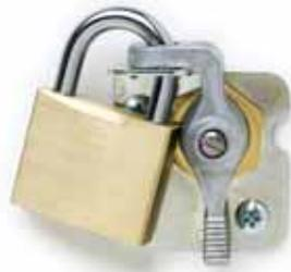
Special lever and flange plate accept a padlock to securely lock a Disconnect Switch in the Off position, which is required by many lock-out/tag-out safety regulations. For use with Cole Hersee lever actuated master disconnect switches with a 3/4" diameter (19.1mm) mounting stem: 2484, 2484-A, 2484-06, 2484-09, 2484-16, 75903, 75904, 75904-01, M-284, M-284-A, M-284-01, M-284-02, M-289, M-290, M-290-01, M-290-05. (We recommend the use of a padlock with a 5/16" (7.9mm) diameter shackle.)
