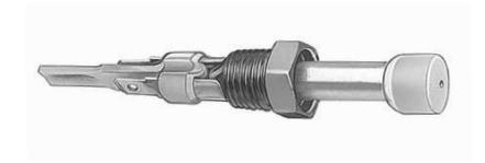
3/8" -24 self-tapping thread, mounting stem .33" (8.38mm) long. Two blade terminals, plunger .85" (21.6mm) long, self-adjusting. 5A at 12V DC.
