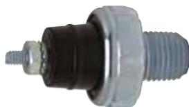
Mounting stem: 1/4" -18 dryseal thread. Normally closed, open at 60 - 70 psi (413.7 - 482.6 kPa). 8-32 stud terminal.
