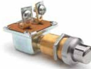
2 screw terminals. Mounting stem: 5/8"-32 thread, 1.06" (26.9mm) long. Gasket seal in the case.
