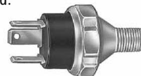
Mounting stem: 10x1mm taper pipe thread. Operation: circuit 1 – terminal 2 normally closed to ground, opens at 4 - 6 psi (27.6 – 41.4 kPa); circuit 2 - terminals 1 & 3 normally open, close at 5 - 7 psi (34.5 – 48.3 kPa).
