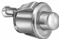
5A at 12V DC. Chrome-plated brass button with chrome-plated faceplate. One bullet terminal. Snaps into 15/16" (23.8mm) diameter hole.
