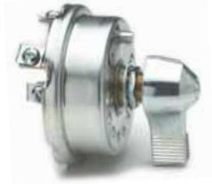
Lever actuator and indexing pin. Four screw terminals. Plated steel case. Mounting stem 1/2"-20 thread. With O-ring seal in the mounting stem. Silver contacts. 30A total at 12V DC.
