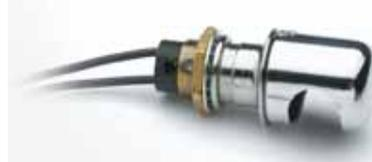
Bright chrome-plated brass hood. 11/16" (17.46mm) diameter mounting stem, 3/8" (9.5mm) long. Bulb not included: suggested lamps: #64 (6V), #68 (12V), #1252 (24V).
