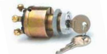
Four brass screw terminals. Diecast case with protective finish. Mounting stem 3/4" -20, 13/16" (20.6mm) long, fits panels up to 1/4" (6.4mm). Knurled aluminum adapter facenut permits mounting in 3/4" (19.1mm) to 7/8" (22.2mm) diameter holes.
