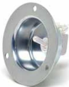
Faceplate only: does not include switch. Needs to be counter-sunk in a 2" (50.8mm) hole. 3 3/16" (81.0mm) diameter with three 7/32" (5.6mm) holes on a 2 3/4" (69.9mm) diameter circle. Requires a clearance depth of .890" (22.6mm), not including clearance for a switch. Other colors, metals and finishes are available on special order. Contact Cole Hersee.
