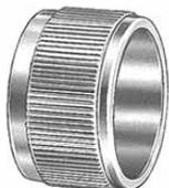
Deep design protects the switch button against accidental operation. Round knurl  $29/32$ " (23.0mm) diameter,  $9/16$ " (14.3mm) thickness.  $5/8$ "-32 thread. Chrome-plated brass.
