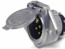
Mounting holes on the flanges are oval, .488" x .328" (12.4 x 8.3mm), 2.93" (74.6mm) on centers. Mounts through 2" (50.8mm) diameter hole.
