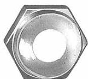
$5/8$ " (15.9mm) hex,  $1/4$ " (6.4mm) thickness.  $3/8$ "-24 thread to fit  $3/16$ " (4.8mm) shaft. Chrome-plated brass.
