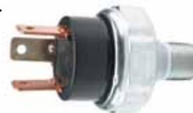
Mounting stem: 1/8"-27 dryseal thread. Operation: circuit 1 – terminal 2 normally closed to ground, opens at 9 - 16 psi (62.1 – 110.3 kPa); circuit 2 - terminals 1 & 3 normally open, close at 9 - 16 psi.
