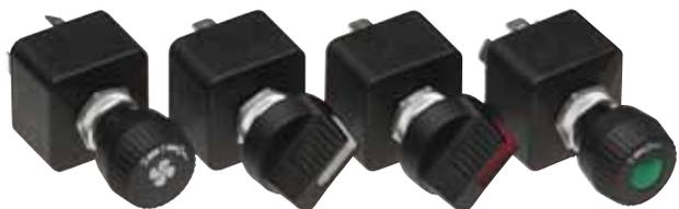
Compact plastic switches, with durable nylon 6/6 body, knob and stem, aluminum hardware, and plated brass terminals. Knobs snap on, and have a very positive detent action. Sealed to IP-53 for protection against dust and contaminants. Terminals accept connectors 99022 or 99021 with standard .250 quick-connect or Faston terminals.
