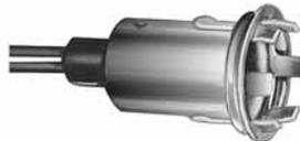
Indexed J slots. Mounting fits 3/4" (19.0mm) diameter hole. Molded plastic insulator. Socket accepts BAZ15d base bulb.
