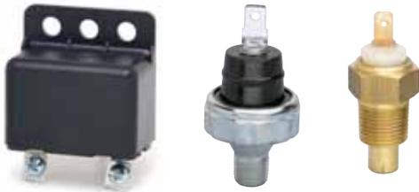
For inboard and outboard engines with 12V DC electrical system. Handy kit includes buzzer 4099, temperature switch 84251, see Section M1, and pressure switch 8606, see Section M3. Alarm sounds when oil pressure is too low and/or engine coolant temperature is too high. Installation instructions included.
