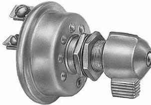
With short diecast lever. Four screw terminals. Plated steel case. Mounting stem 5/8"-32 thread. With O-ring seal in the mounting stem. 20A per circuit at 12V DC.
