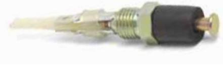
3/8" -24 thread, mounting stem 7/32" (5.6mm) long. Two blade terminals, plunger 3/16" (4.8mm) long, self-adjusting to 1/4" (6.4mm) long. Operates with 7lbs (3.2 kg) minimum pressure. 5A at 12V DC.
