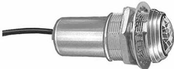
12V #67 bulb supplied. 15/16" (23.8mm) diameter lens, gasket-sealed. 7/8" (22.2mm) diameter mounting stem, 3/4" (19.1mm) long. Plated brass bezel, 1 1/4" (31.8mm) diameter. Faceted outer lens surface.
