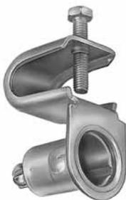
Plated steel clamp. Screw terminals. Molded plastic insulator. Socket accepts BA15d base bulb.
