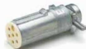
Diecast housing, polarized ground terminal, insulated. Replacement for ISO 3731-1976 (E) road vehicles, type 24S (supplementary). Contacts: six spring-grip female, and one solid male pin. Mates with Cole Hersee 12077-01 ISO socket.
