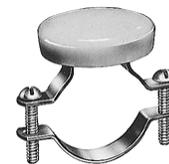
5A at 12V DC. Two screw terminals. Ivory plastic button 1 3/4" (44.5mm) diameter. Clamp allows attachment on a steering column up to 1 1/2" (38.1mm) diameter.
