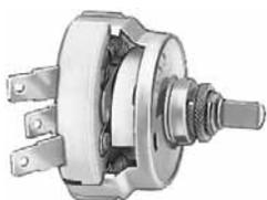
2 Ohm rheostat with 22W rating. Off - On 1 - On 1, 2 High - On 1, 2 Low. 7/16" -28 thread mounting stem, .25" (6.4mm) long. Three blade terminals. Plated steel case, 1.78" (44.6mm) diameter, .875" (22.2mm) long. Without knob.
