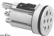
For 12301 plug. Glass-filled plastic insulator, spring-grip brass contacts. O-ring seal.
