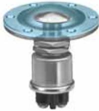
35A at 12V, 20A at 24V DC. Picture shows typical vertical mounting location. Mounting plate and diaphragm are not supplied. Off-Momentary On, spring return to Off. Brass case and mounting hardware. Silver contacts. Two brass screw terminals. Brass mounting stem 5/8"-32 thread, 7/16" (11.1mm) long, fits panels up to 3/16" (4.8mm) thick. Anodized aluminum button 15/16" (23.8mm) diameter. Plunger button is loose, and must be held in place with rubber diaphragm.
