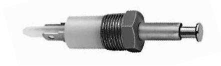
1/2" -28 self-tapping thread, mounting stem 5/16" (8.0mm) long. Two blade terminals, plunger 3/4" (19.0mm) long, self-adjusting to 9/16" (14.3mm) long. 5A at 12V DC.
