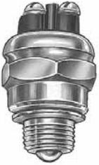
20A at 12V DC. Two-screw terminals. Mounting stem 3/4" -16 UNF-2A thread, 31/64" (12.3mm) long.
