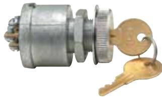
Four screw terminals. Diecast case. 3/4" -20 mounting stem, fits panels up to 1/2" (12.7mm).
