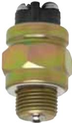
Two screw terminals. Mounting stem 3/4" -16 UNF-2A thread, 31/64" (12.3mm) long, with aluminum gasket/washer. Replaces: Clark 224620
