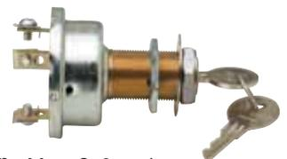
10A at 12V DC. Mom On1 - Off - Mom On2, spring return to Off from both positions. Key actuator with coded tumblers lock. Mounting stem 13/16"-24 thread. Internal O-ring seal.
