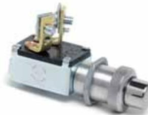
15A resistive, 10A inductive at 12V DC, 8A resistive, 5A inductive at 24V DC. Two screw terminals. Mounting stem: 5/8"-32 thread, .87" (22.1mm) long.
