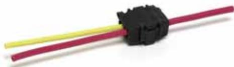
Use Quick-Tap to connect two wires or create a tap without stripping the wires. Two wires can be connected in-line or as a pigtail. Consists of a small molded plastic hinge unit. Insert the wires, close and snap shut with pliers. Fully insulated to prevent short circuits. Splicing instructions are included. 10 per pack.
