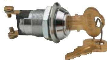
Electrical ratings at 12V DC: 5A Ignition. Two brass screw terminals. Brass case with chrome-plated integral bezel. Brass mounting stem 3/4" -27, 3/4" (19.1mm) long, fits panels up to 5/8" (15.9mm). Double bit keys.
