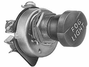
Illuminated tan knob with 'Fog Light' imprint. Three screw terminals. Plated steel case. Mounting stem 5/8"-32 thread. 20A fuse and No. 53 bulb supplied.
