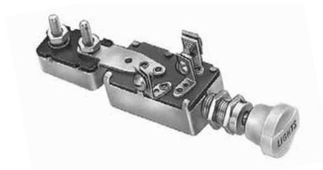
With 30A at 12V circuit breaker, ivory knob imprinted 'Lights'. Three screw terminals, plated steel case, silver contacts, mounting stem with 7/16"-28 thread.
