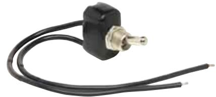
Moisture- and dirt-resistant. PVC coated and sealed with an O-ring seal in the stem. Up: Off, Down: Mom On. Two 8" (203.2mm) leads.
