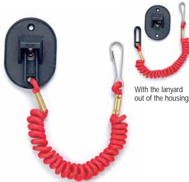
With the lanyard out of the housing.
