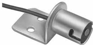
Plated steel bottom bracket, with two 13/64" (5.2mm) holes, 1/2" (12.7mm) on centers. Socket accepts BA15s base bulb.
