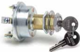
15A at 12V DC. Key actuator with coded tumbler lock. Spring return to Off from both On positions. O-ring seal in stem. Mounting stem 13/16"-24 thread.
