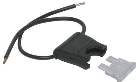
Accepts ATO and ATC fuses and circuit breakers from 3A to 20A. Easy to install and easy to change the fuse. 16AWG insulated copper wire leads, 4" (101.6mm) long. Brass contacts. Supplied without a fuse.
