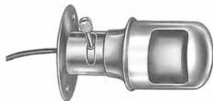
Bright chrome-plated brass hood with wide aperture. Flange mounting, with two 9/64" (3.6mm) diameter mounting holes, 1 3/16" (30.2mm) on centers. Bulb not included. Suggested lamps: #63 (6V), #67 (12V), #623 (24V). Integral On-Off switch in the stem.
