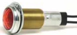
15/16" (23.8mm) diameter lens, gasket-sealed. Plated brass bezel, 1 1/4" (31.8mm) diameter. 7/8" (22.2mm) diameter mounting stem, 1 1/4" (31.8mm) long. 12V #68 bulb supplied. Moisture-repellent insulator.
