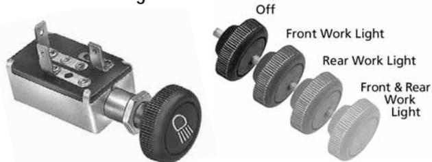
Three blade terminals. Plated steel case. Mounting stem 7/16"-28 thread. With O-ring seal at the mounting stem. With black knob imprinted with SAE work light symbol.
