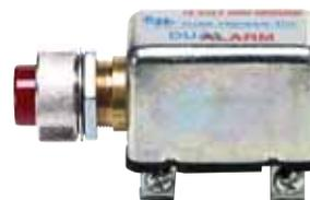
Rugged combination warning light and buzzer give audible and visible alert. Universal application: use with any electrical switch. Red lens, long-life LED. 11/16" (17.46mm) diameter mounting stem, 17/32" (13.88mm) long. Body size: 1 7/8"L x 1"W x 1 11/32"H ( 47.6 x 25.4 x 34.1mm). Wiring instructions provided. 12V DC. Also available as 24V. Item No. 4124-RD.
