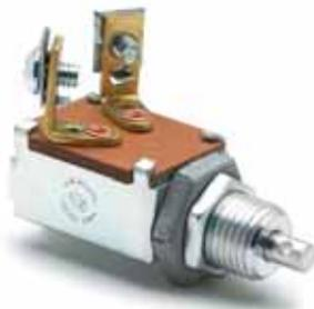
10A at 12V DC. Normally Off. Pull On, spring return to Off. Brass case and mounting hardware. Two screw terminals with lockwashers. Mounting stem 1/2"-20 thread, 5/8" (15.9mm) long. No knob: shaft has 3/32" (2.4mm) hole for the attachment of a cable or lever.
