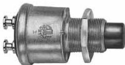
Two male button head terminals, accept Delphi (Packard) connector 2962679, or equivalent. Mounting stem: 5/8"-32 thread, 5/8" (15.9mm) long. Accepts screw-on protective cap 83280-03. Black plastic button.
