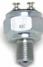
15A at 12V DC. Two-button head accepts standard female blade terminals, and will mate with Delphi (Packard) 2-pole connector 2962679, or equivalent. Mounting stem 9/16" -18 UNF-2A thread, 21/32" (16.7mm) long.
