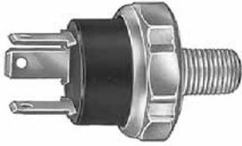
Mounting stem: 10x1mm taper pipe thread. Operation: circuit 1 – terminal 2 normally closed to ground, opens at 2 - 6 psi (13.8 – 41.4 kPa); circuit 2 - terminals 1 & 3 normally open, close at 9.5 psi or less (65.5 kPa).
