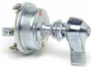
15A at 12V DC. Lever actuator. Silver contacts. Mounting stem 1/2"-20 thread, 1 1/4" (31.8mm) long.
