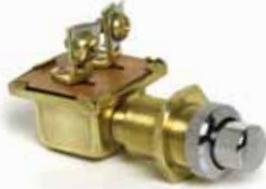
Two brass screw terminals. Brass mounting stem 5/8"-32, 1" (25.4mm) long. Fits panels up to 3/4" (19.1mm) thick. Gasket-sealed case.
