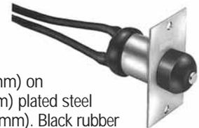
Two .144" (3.7mm) diameter mounting holes, 1 1/2" (38.1mm) on centers. 0.70" diameter (17.8mm) plated steel case. Plunger: 0.436" long (11.1mm). Black rubber cap on plunger, and PVC coating on 8" (203.0mm) wire leads protect against moisture and dirt. 5A at 12V DC.
