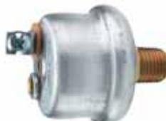
Mounting stem: 1/4" -18 dryseal thread. Normally closed, open at 60 - 70 psi (413.7 - 482.6 kPa). 8-32 screw terminal.
