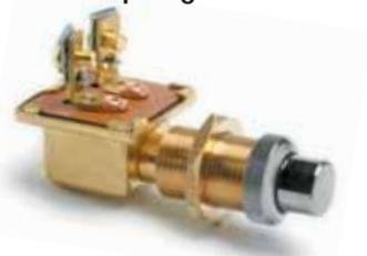
Chrome-plated brass plunger. Two brass screw terminals. Brass mounting stem 5/8"-32 thread, 1" (25.4mm) long. Fits panels up to 3/4" (19.1mm) thick.
