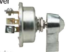
20A at 12V DC. Lever actuator, spring return to Off from both On positions. Silver contacts. Mounting stem 7/16"-28 thread.
