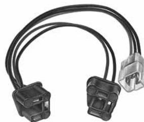
For Chevrolet and GMC RVs. Accepts one 3-prong headlamp and one 2-prong headlamp. This harness attaches to a 3-pole Packard connector that is supplied with the vehicle chassis. Leads are 16AWG wire that connects into silvered bronze contacts in molded plastic connectors.
