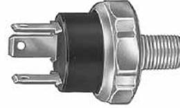
Mounting stem: 3/8"-18 dryseal thread. Operation: circuit 1 – terminal 2 normally closed to ground, opens at 4 - 7 psi (27.6 - 48.3 kPa); circuit 2 – terminals 1 & 3 normally open, close at 6 - 9 psi (41.4 - 62.0 kPa).
