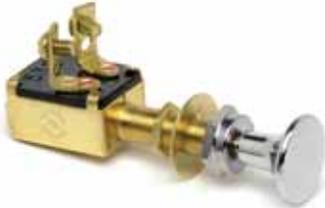
10A at 12V DC. Normally Off. Pull On, spring return to Off. Brass case and mounting hardware. Two brass screw terminals. Brass mounting stem 3/8"-32, 1 1/4" (31.8mm) long. Fits panels up to 7/8" (22.2mm) thick. Chrome-plated brass knob, debossed 'PULL', 7/8" (22.2mm) diameter. Moisture-repellent insulator.
