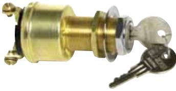
Four brass screw terminals. Brass case and mounting hardware, chrome-plated brass facenut. Brass mounting stem 13/16" -24, 1 7/32" (31.0mm) long, fits panels up to 1" (25.4mm).
