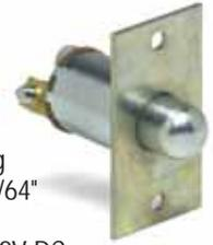
Two screw terminals. Two 9/64" diameter (3.6mm) mounting holes, 1 3/8" (34.9mm) on centers. 45/64" diameter (17.9mm) plated steel case. Plunger: 7/16" long (11.1mm). 5A at 12V DC
