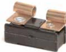
Breaker replaces 3AG (AGC) and SFE glass fuses: snaps into standard clips on Cole Hersee fuse blocks. See section H3. Available in 10, 15, 20, 25, 30, 40A. Order Nos. 30410-40 etc. 10A replaces Ford DOHB-14526-A, 15A DOVB-14526-A, 20A DOVB-14526-B, 25A DOHB-14526-B, 30A DOVB-14526-C.
