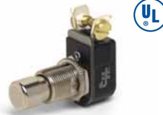
6A at 125V, 3A at 250V. Push On, spring return to Off. For AC or DC. UL-approved. Plastic body, nickel-plated plunger. Two screw terminals. 15/32" -32 mounting stem, 9/16" (14.3mm) long.
