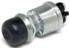
Two screw terminals. Mounting stem: 5/8"-32 thread, 21/32" (16.7mm) long. With screw-on black rubber protective cap 83280-03.
