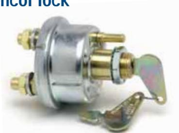
Mounting stem: Brass, 3/4" -16 thread 17/32" (13.5mm) long. Fits panels up to 1/4" (6.4mm) thick. Terminals: Two 3/8" -24 studs. Plated steel case, silver-laminated contacts. Hencol lock and 2 keys. Indexing pin.
