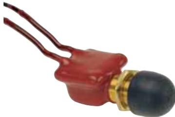
PVC-coated body sealed against moisture and dirt, with black rubber snap-on cap 407-03. Two 12" (304.8mm) 18AWG leads. Brass mounting stem 5/8"-32, 15/16" (23.8mm), fits panels up to 1/2" (12.7mm) thick.
