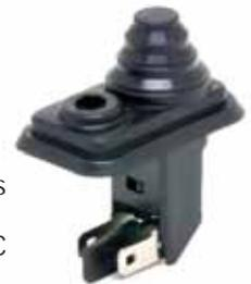
Black rubber boot covers and protects the face of the switch, making it dust-resistant. Plastic button. 4A at 12V DC lamp load. Two 2mm x 5mm blade terminals. 4A at 12V DC.
