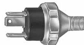
Mounting stem: 1/8"-27 dryseal thread. Operation: circuit 1 – terminal 2 normally closed to ground, opens at 2 - 8 psi (13.8 – 55.2 kPa); circuit 2 - terminals 1 & 3 normally open, close at <11 psi (75.9 kPa).
