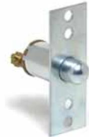
Four 3/16" diameter mounting holes, 1 3/8" and 2 1/16" on center (34.9, 51.0mm). 45/64" diameter (4.8mm) plated steel case. Plunger: 7/16" long (11.1mm). 5A at 12V DC.
