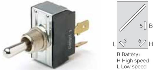
Double pole, two-circuit. Three blade terminals. Up: Battery & High - Center: Battery & Low - Down: Off. Standard handle. Terminal connections: 3 low speed, 5 Battery +, 6 high speed.
