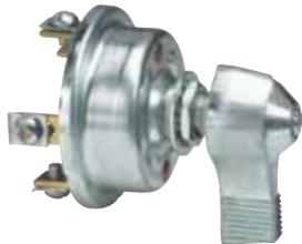
15A at 12V DC. Lever actuator. Silver contacts. Mounting stem 1/2"-20 thread, 13/32" (10.4mm) long.
