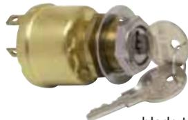
Key is removable only in the Off position, spring return to IGN. Electrical ratings at 12V DC: 5A Ignition, 5A Start, 2A Choke. One brass screw and three brass blade terminals. Brass case and mounting hardware, chrome-plated brass facenut. Brass mounting stem 13/16" -24, 15/16" (23.8mm) long, fits panels up to 1/2" (12.7mm). O-ring seal in the mounting stem.
