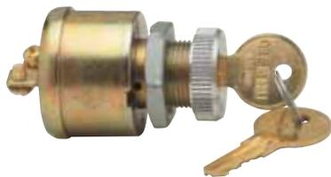
Three brass screw terminals. Diecast case with protective finish. Mounting stem 3/4" -20, 13/16" (20.6mm) long, fits panels up to 1/4" (6.4mm). Knurled aluminum adapter facenut permits mounting in 3/4" (19.1mm) to 7/8" (22.2mm) diameter holes.
