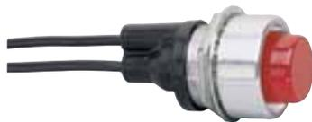
Mount from the front of the panel, fasten from the back. Satin finish or black aluminum bezel, 15/16" (23.8mm) diameter. 12V #1893 bulb supplied. 5/8" (15.9mm) diameter lens. 3/4" (19.1mm) diameter mounting stem, 3/8" (9.5mm) long. Available with custom imprinting: contact Cole Hersee.
