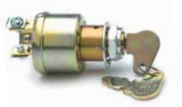
Three screw terminals. Plated steel case. 5/8" -32 mounting stem. O-ring seal in mounting stem. Fits panels up to 9/16" (14.3mm) thick.
