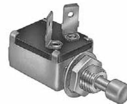
2 blade terminals. Mounting stem: 7/16"-20 thread, 1/2" (12.7mm) long. 1/2" (12.7mm) plunger with nylon cap.
