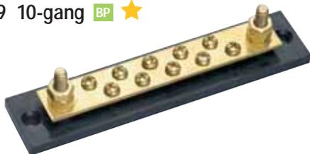
Solid brass busbar safely carries up to 150A. Two 1/4-20 brass studs with hexnuts. 8-32 round head screws for attachment of wires. Two mounting holes accept No.10 countersink flat-head screws. Moisture-resistant molded thermoplastic insulator base. 5 3/4"L x 1 1/4"W x 1 1/32"H (146.0 x 31.7 x 26.1mm). Two mounting holes 5.19" (131.8mm) on centers.
