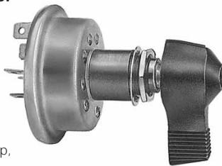
With black nickel-plated lever actuator. Five blade terminals, accepts Delphi (Packard) connector 2962912. Plated steel case. Mounting stem 5/8"-32 thread. With O-ring seal in the mounting stem. 20A per circuit at 12V DC.
