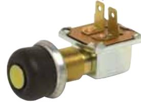
Two blade terminals accept 2-pole Delphi (Packard) connector 2977647 or equivalent. Mounting stem: 5/8"-32 thread, .625" (15.9mm) long. Gasket seal in the case. Steel plunger protrudes through the cap. Black rubber cap snaps into a special groove on the nut, which is deep-threaded and gives a positive seal.
