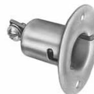
Flange has two 9/64" (3.6mm) holes, 1 3/16" (30.2mm) on centers. Screw terminals, molded plastic insulator. Socket accepts BA15s base bulb.
