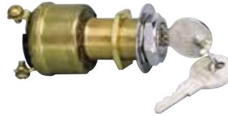
Three brass screw terminals. Brass case and mounting hardware, chrome-plated brass facenut. Brass mounting stem 13/16" -24, 1 7/32" (31.0mm) long, fits panels up to 1" (25.4mm).
