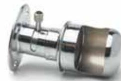
Bright chrome-plated brass hood. Flange mounting, with two 9/64" (3.6mm) diameter mounting holes, 1 3/16" (30.16mm) on centers. Two screw terminals. Integral On-Off switch in the stem. Bulb not included: suggested lamps: #64 (6V), #68 (12V), #1252 (24V).
