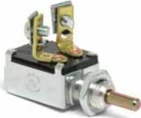
7/16" -20 thread mounting stem, 7/16" long (11.1mm), two flats on stem for mounting in double-D hole. Two screw terminals, plated steel case. 10A at 12V DC.
