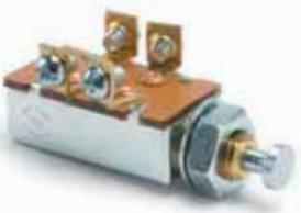
7/16" -20 thread mounting stem, 7/16" (11.1mm) long, two flats on stem for mounting in double-D hole. Four screw terminals. Plunger 19/64" (7.54mm) long. 10A at 12V DC.
