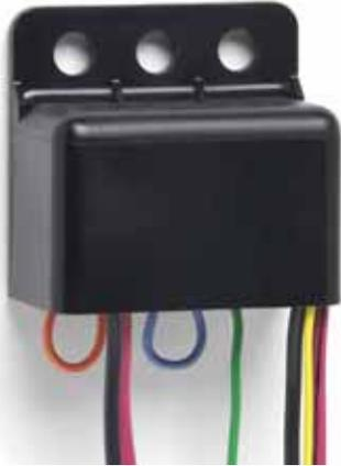
**Wiring:** 2 power in, 2 power out, control wire to momentary switch. Instructions are included. Power wires 16AWG control wires 18AWG, loops 22AWG. System voltage 12V DC (9-16V).
