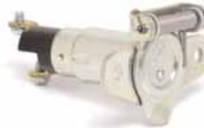
Plated steel housing. Molded plastic insulator. Cover locks firmly in place when not in use. Two .20" (5.2mm) diameter mounting holes, 1.87" (47.4mm) on centers.
