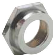
$7/8$ " (22.2mm) hex,  $15/64$ " (6.0mm) thickness.  $13/16$ "-24 thread to fit  $5/8$ " (15.9mm) shaft. Chrome-plated brass.
