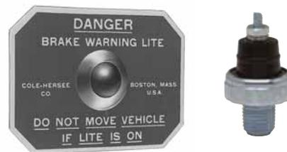
Lamp flashes when pressure switch triggers at 60+10 psi (413+69kPa). Includes heavy duty Air Pressure Switch 8640 (has 1/4-18 NPTF thread). Aluminum faceplate with red enamel finish, 2.94"W x 2.09"H (74.7 x 52.1mm). Pilot light with flashing bulb. Two 16AWG wire leads, one 18" (457.2mm) and one 8" (203.0mm). Installation instructions included.
