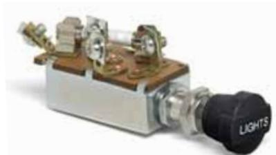
With 20A at 12V glass fuse, black knob imprinted 'Lights'. Four screw terminals, plated steel case, mounting stem with 7/16"-28 thread.
