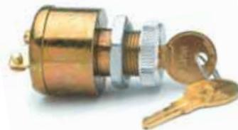
Electrical ratings at 12V DC: 10A Ignition. Two brass screw terminals. Diecast case with protective finish. Mounting stem 3/4" -20, 13/16" (20.6mm) long, fits panels up to 1/4" (6.4mm). Knurled aluminum adapter facenut permits mounting in 3/4" (19.1mm) to 7/8" (22.2mm) diameter holes.
