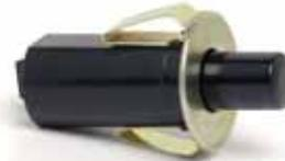
Snaps into .80 - .85" (20.3 - 21.6mm) diameter hole. Fits panels .03 - .07" thick (.76 - 1.8mm). Moisture-resistant molded plastic case. Two female bullet terminals, plastic plunger 9/16" (14.3mm) long.
