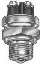
35A at 12V DC. Two female bullet terminals. Mounting stem 3/4" -16 UNF-2A thread, 31/64" (12.3mm) long. Replaces: Chrysler 1527835, Clark 73631.
