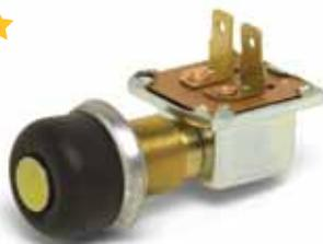
20A at 12V DC, 10A at 24V DC. Silver contacts. Rubber cap snaps into special groove and is secured to the mounting stem by a deep-threaded nut for a positive seal. Two blade terminals mate with two-pole Delphi (Packard) connector 2977647 or equivalent. 5/8" -32 thread mounting stem, .625" (15.9mm) long. Gasket-sealed case. Steel plunger protrudes through the cap.
