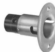
Flange has two 9/64" (3.6mm) holes, 1 3/16" (30.2mm) on centers. Screw terminals, molded plastic insulator. Socket accepts BA15s base bulb.
