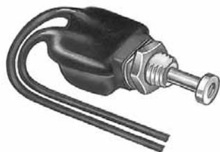
10A at 12V DC. Plasticized housing protects against moisture and dirt. Two 18AWG wire leads, 7" long. Button-head actuator, 3/8" (9.5mm) long. 7/16" -20 (7.9mm) diameter mounting stem with two flats for mounting in double-D holes. Replaces: AMC 3171244.
