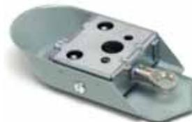
Attaches to a cord. For use by passengers in buses and rapid transit vehicles. Extra heavy duty construction. Use with Cole Hersee buzzers or buzzer/flashers: 4099, 4112 RC, 4124-RD. SPST Off-Mom. On. Normally Off, pull to On, spring return to Off. For use with systems up to 36V DC. Two screw terminals. Neutral gray enamel finish cover. Operates with a pull cord.
