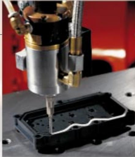
A robust, 100% solids silicone, FastGasket® is dispensed with precision and repeatability by programmable, robotic tracing equipment directly into the surface groove of the most complex flanges. Each year, more than fifteen million of these cured-in-place (CIP) gaskets seal flanges in vehicles worldwide.
