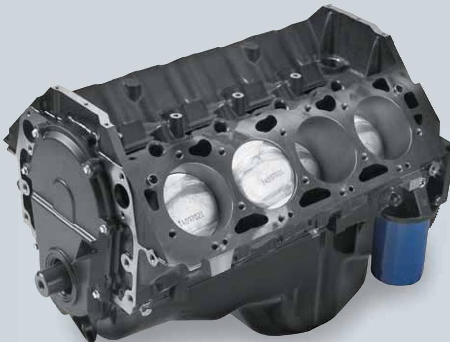
For those who want the sturdy foundation of the ZZ454 as the starting point of a custom engine, this brand-new partial engine includes the forged crank, rods and pistons, as well as the balancer, oil pan and front cover. This partial engine does not include a camshaft, lifters, timing chain or cam sprocket. All parts necessary to complete the engine are available from your GMPP dealer. Use externally balanced flywheel for manual transmission applications.
