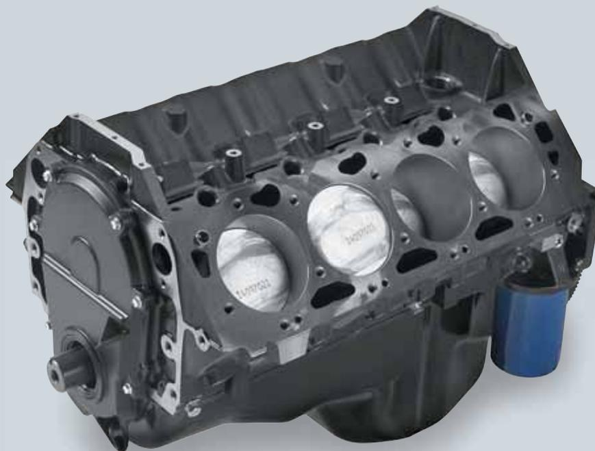
For those who want the sturdy foundation of the 454 HO as the starting point of a custom engine, this brand-new partial engine includes the forged crank, rods and pistons, as well as the balancer, oil pan and front cover. This partial engine does not include a camshaft, lifters, timing chain or cam sprocket. All parts necessary to complete the engine are available from your GMPP dealer. Use externally balanced flywheel for manual transmission applications.
