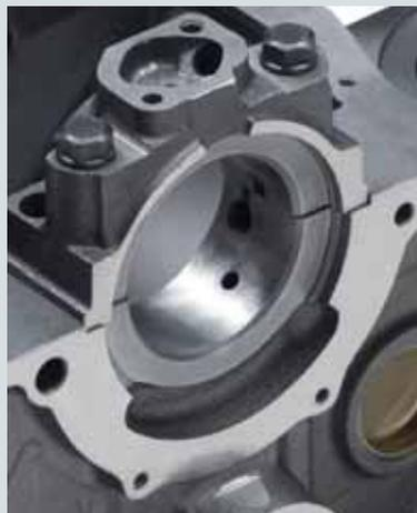
**A** Two-Bolt Rear Main (no seal adapter)
