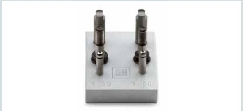
**D** Rocker Arm Ratio Checking Tool
