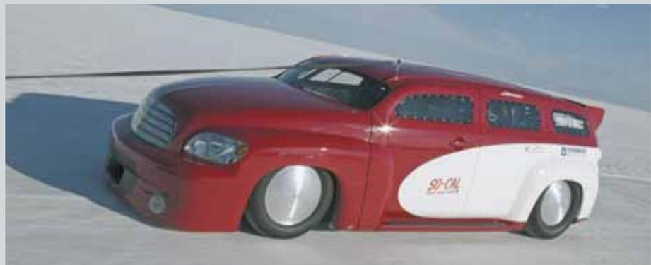
impressive, and assembled by four female engineering students. It went 140 mph in testing and is powered by 230 horsepower version of a turbocharged 16-valve Ecotec four cylinder.
