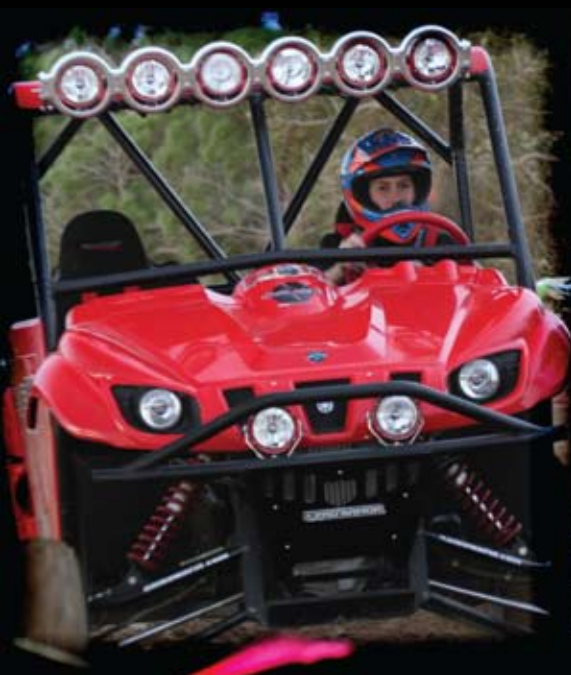
Above: UTV Dual Fuego Light Kit - Attached Using Welded Bumper Tabs.
