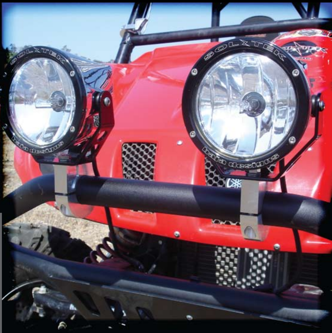
Above: UTV Dual Fuego Light Kit - Attached Using Welded Bumper Tabs.
