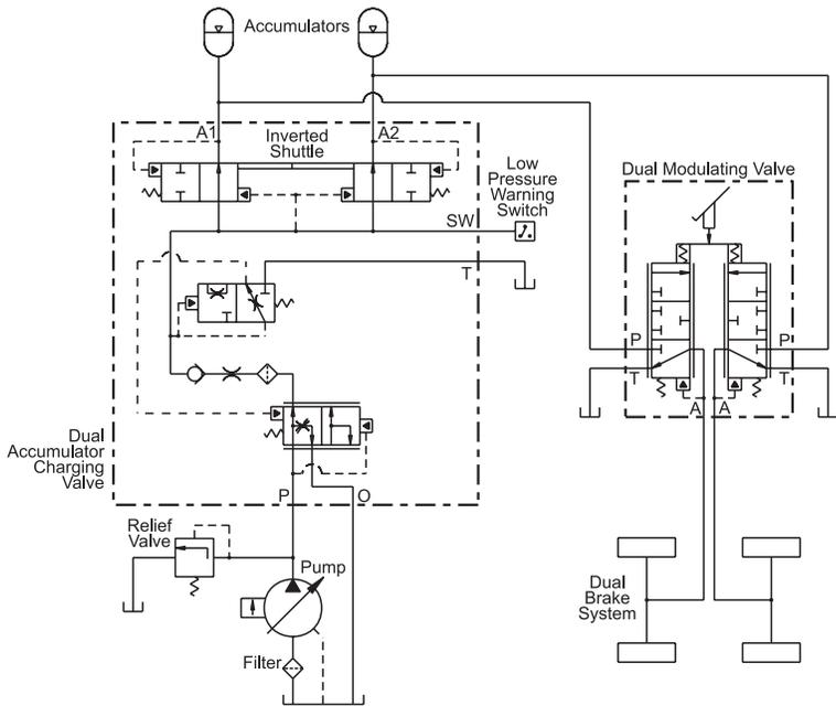
**Dual Closed Center Brake Circuit in a Non-Dedicated Load Sense Hydraulic System**
