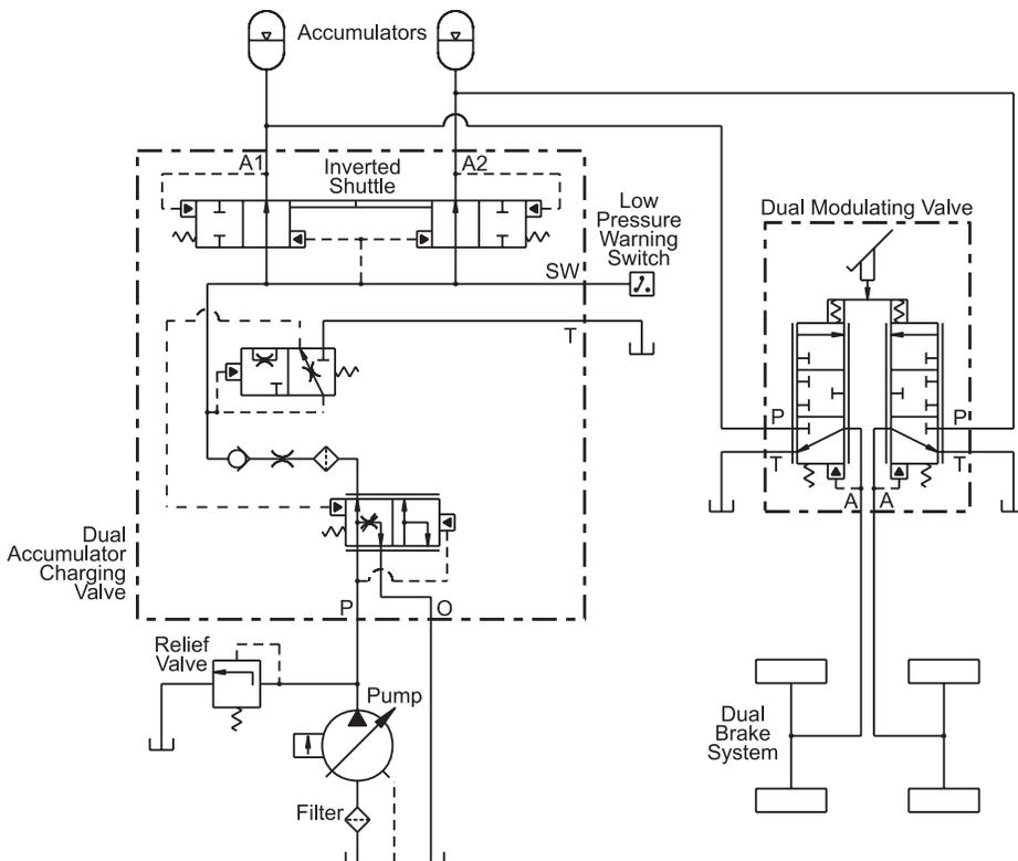
**Dual Closed Center Brake Circuit in a Dedicated Open Center Hydraulic System**
