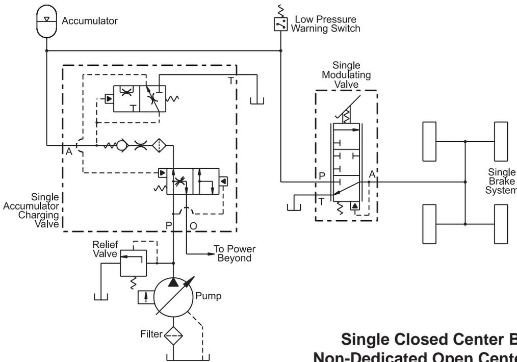
**Single Closed Center Brake Circuit in a Non-Dedicated Open Center Hydraulic System**
