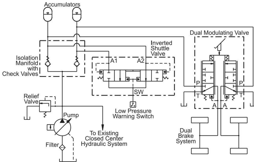
**Dual Closed Center Brake Circuit in a Non-Dedicated Closed Center Hydraulic System**
