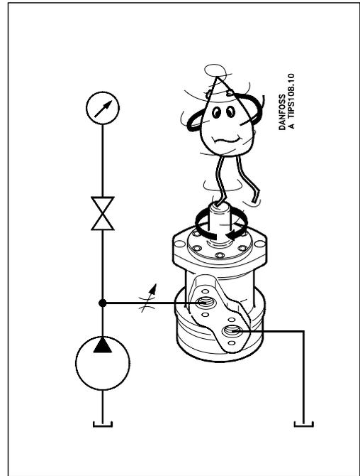
If no flow meter is available, a Danfoss hydraulic motor can be fitted instead. The displacement of the motor per revolution with unloaded shaft is very precise and to find flow all that is necessary is to count the number of revolutions per minute and multiply the figure by the displacement, as shown in the following examples:
