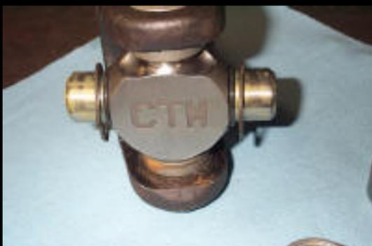
When you have finished installing both snaprings and clips, the cross should rotate freely in the bearing caps with no hint of bind, but you shouldn't be able to spin either snapring in its groove just by trying to turn them with your fingers
