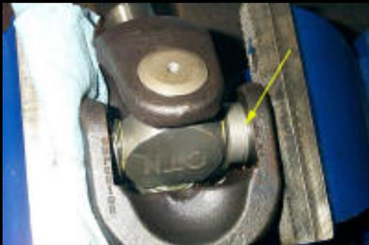
8. Continue to press the cap on until the snapring groove (yellow arrow) is fully inside the yoke.
