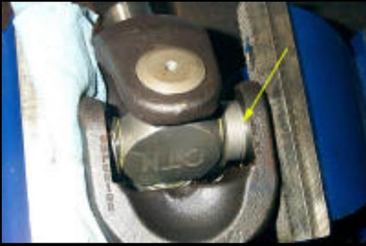
17. Stop when the snapping groove is inside the yoke
