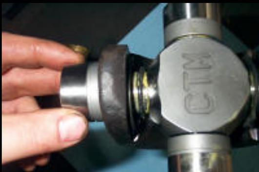
5. Carefully install a bearing cap on the trunnion by pressing it through the hole in the axle yoke.
