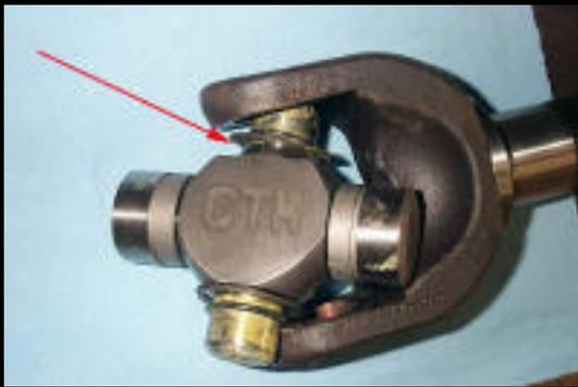
2. Hold the cross so the CTM label faces you and the cut-out is at the top facing you. Place the snapping in the cut out area (red arrow) and slip this trunnion into the yoke first.
