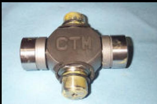
1. Take a joint, remove a pair of opposing bearing caps, and onto each trunnion place a snapping followed by an o-ring.
