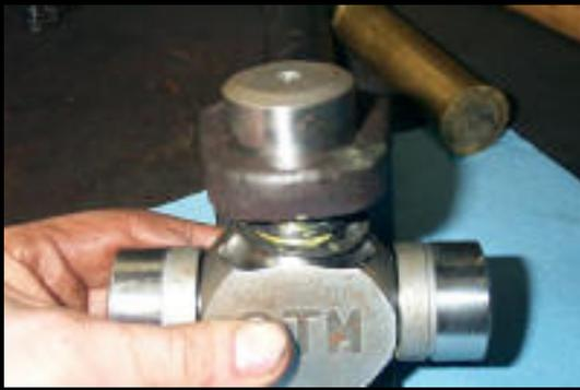
Start by using your fingers, being extra careful to keep the trunnions, caps, and yoke bores all lined up, and making sure the o-rings and snaprings aren't pinched or caught up...
