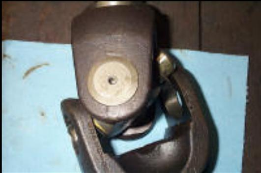
15. The trickiest part of the CTM installation is getting the cross in the second yoke. Because of the size of both the U-joints and the Superior Alloy shafts clearances are quite tight. You will have to carefully align the trunnions with the yoke bores...
