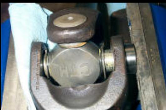
16. Once the cross is situated in the yoke of the second axle, proceed as above to press on the first cap
