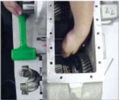
11. Remove the shift forks. If you are doing a shift fork upgrade only, move to procedure 20. **Note:** Atlas cases #1929 & earlier are the only units that need to have shift fork upgrades.
