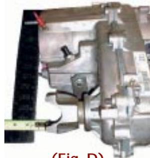
**FRONT MEASUREMENT:** Measure the stock transfer case from the front yoke face to the surface of where the transfer case bolts to the adapter housing (Fig. D). Write that measurement down.
