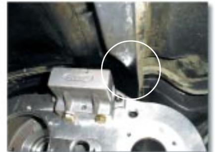
Upper body modification for clearance when the Atlas is rotated shallower than stock.
