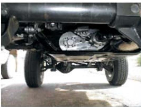
If you plan on using a lift kit in addition to your new Atlas, it is important that you correct your pinion angle when running a rear C.V. type driveshaft. The pinion angle should be equal to that of the output driveshaft. Many aftermarket suspension systems allow you to adjust the lower control arm length to give you the pinion angle you need.
