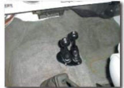
The Atlas twin stick is designed as a universal application. We recommend [Part No. 303001R](#) for the correct shifter configuration. This shifter protrudes 5-1/2" from the face of the Atlas, but is easily shortened to other lengths. Both handles on the shifter are straight and fit in the vehicle side-by-side. As long as your CJ is not equipped with an aftermarket console, the shift handles should have adequate clearance.
