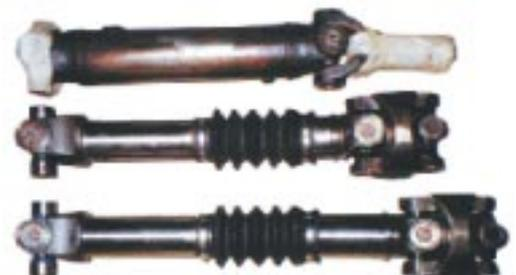
Stock driveshaft (top) vs. new fixed yoke driveshafts
