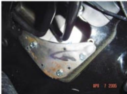
The sticks will come up through the stock floorboard hole. You will be required to cover a small portion of the stock hole. The rear driver's side will need a piece of sheet metal to be added. **Make sure the handles move freely and don't touch the floorboard. Interference will cause the unit to pop out of gear.**
