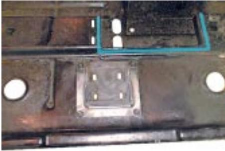
No matter which option you decide to do, we recommend that you provide clearance on the crossmember for the Atlas drain plug. This drain plug is located on the access pan of the transfer case.
