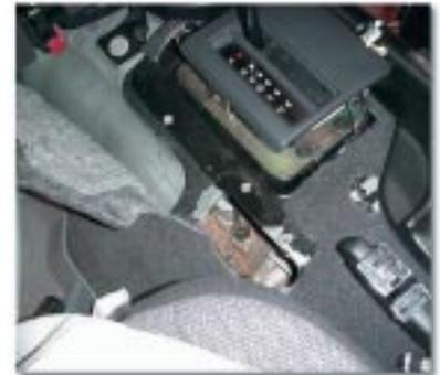
This photo shows the Jeep console removed and the transfer case linkage removed.
