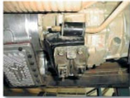
The modified transmission bracket with the rubber support in the new location.
