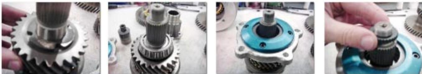
16. Take the new front assembly and turn it over (as shown below) and install the caged needle bearing for the low gear on the shaft. Insert the new assembly into the Atlas case. As the front assembly is being installed, slip the low gear onto the rear portion of the shaft and onto the needle bearing.
