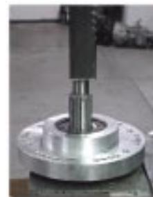
Once the gear is removed, the input shaft can also be removed. Since the input shaft is a press fit onto the front bearing, the shaft is pressed out as shown above.
