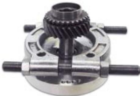
The drive gear is a light press fit onto the input shaft. It is required to be pressed off for disassembly and pressed on for assembly.
