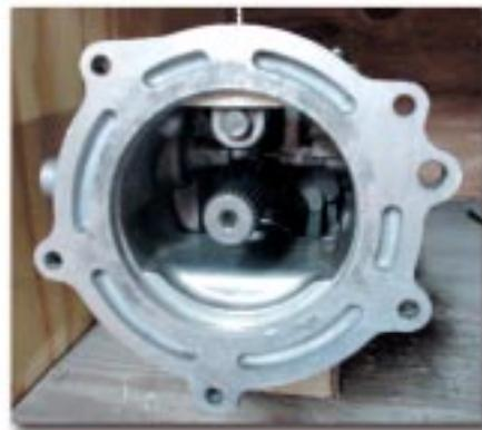
Photo of a stock Ford tailhousing. All Ford Explorers, Rangers, and Bronco IIs have the same bolt pattern and splines when coupled to a 1350 transfer case. The adapters we manufacture for these vehicles to fit the C4 and AOD would also have this same pattern.
