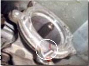
We have provided (5) 10-1.5mm x 35mm long bolts in the Explorer shifter kit for the transfer case-to-transmission adapter. Due to different adapter thicknesses, make sure that these do not bottom out in the Atlas case when tightened. You will be required to remove the stock breather hose bracket from the stock tailhousing because it will interfere with the Atlas shifters.
