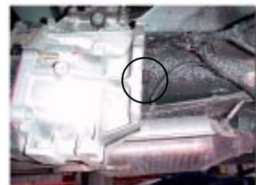
AX5 should have 1/2" output shaft stickout.
