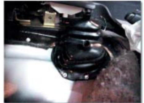
Test fit the Atlas shift handles. If proper clearance has been obtained, screw the rubber boot and ring to the floorboard. Note: The boot ring will need to be cut in half for proper fit to your floorboard.
