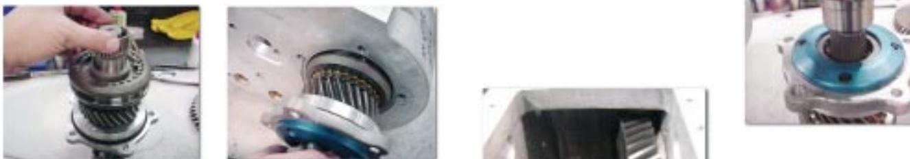
17. With the front assembly further into the case, install the original spacer and the original tapered bearing. This assembly will then pilot into the bearing race located in the back of the transfer case.
