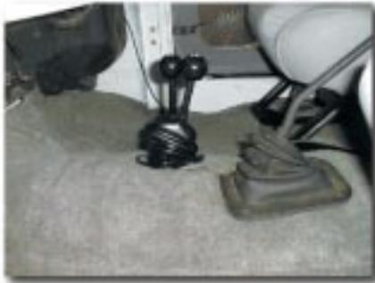
On some CJs, Jeep used an indicator light for 4WD. The Atlas has provisions to use a late model 4WD indicator switch found in the stock "TJ" models, Jeep Part No. J8134473. On average, this part is priced around \$20.00. If you prefer not to use the indicator, use the plug included in your kit.
