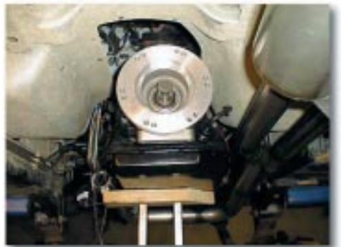
By unbolting and removing your stock transfer case, you should have your transfer case adapter and output shaft exposed. The adapter housing transfer case mating flange should be cleaned of any debris. Double check the output shaft splines of your transmission and verify the stickout length. Make sure the Atlas has the same spline and that the length of the transmission output isn't too long for the Atlas input. (Refer to the Atlas Input Shaft section for more information).
