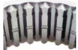
This photo shows the taper of the splines on the shifter slider.
