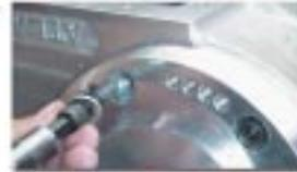
Remove the 6 Atlas input ring bolts and remove the input ring assembly from the transfer case.
