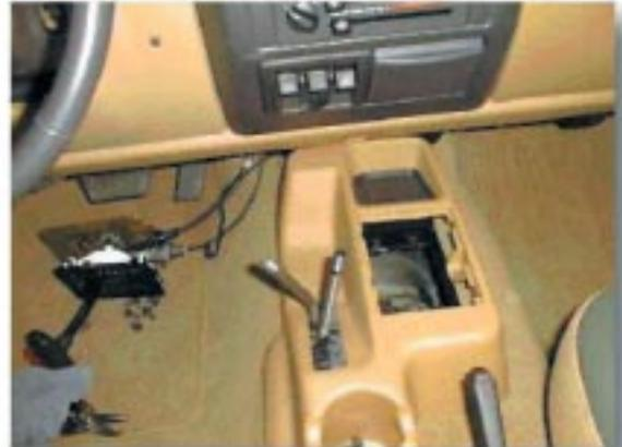
Place the stock console in its original position to test fit the Atlas handles. Rotate the twin stick assembly so that it aligns with the console slot. Once the correct position is obtained, remove the console again.
