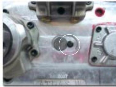
you will need to remove the cluster pin bolts from both the front and rear of the transfer case (photos shown right & left). From the front of the transfer case, push the cluster pin out of the case. You should be supporting the cluster gear with one hand as you push out the cluster pin with the other.
