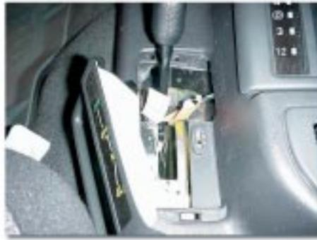
The stock console will require disassembly and the stock transfer case linkage will need to be removed.
