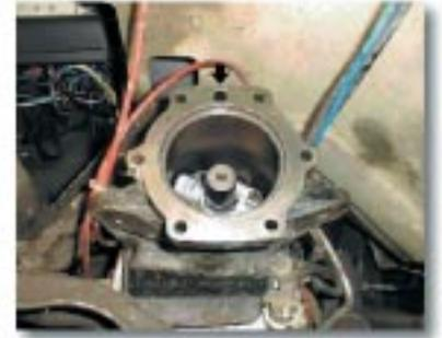
contact us for the necessary machining specifications or for a replacement housing. When removing the stock transfer case and exposing the tailhousing adapter, you'll also find that Ford used a large dowel pin located at the top of the stock housing (shown above left). This dowel pin must be removed (shown above right).
