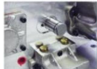
6. Remove the cluster gear. **Note:** Use special care not to drop the bearings from inside the gear.
