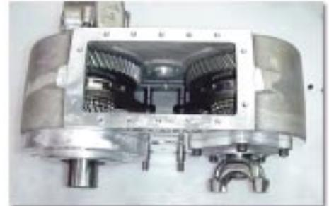
22. Install the cluster gear, thrust bearings, and cluster pin. Two new o-rings have been provided for the cluster pin. Be careful to make sure that the thrust washers are properly aligned between the inside of the case and cluster gear.
