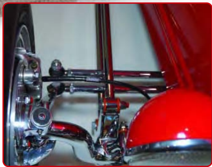
Russell Universal Black Brake Hose installed on Edelbrock's '32 Ford Highboy Roadster
