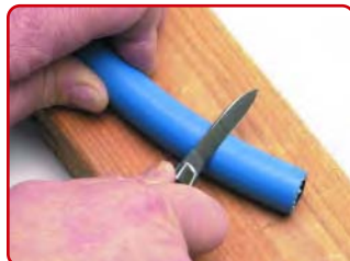
Step One: Cut hose to length using a sharp knife or shears.
