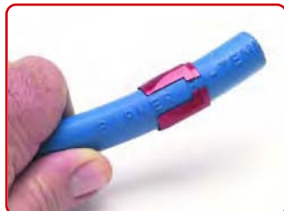
Step Two: Slide decorative red socket over hose (the hex end goes toward the tip of the hose). Liberally oil the inside of the hose and barbed end of the hose end.
