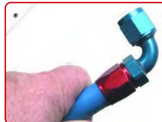
Step Four: Using a flat screwdriver, pry the hex socket open and push up until it bottoms out on the hex. Note: Be sure the slot is positioned to the back of the hose assembly for appearance purposes.
