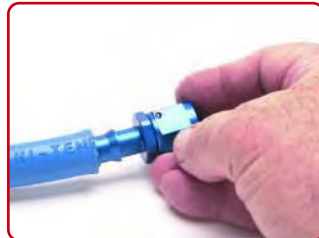
Step Three: Insert the barbed end into hose using a twisting action. Put the swivel end at center hex in a vise. Use a twisting motion make the bottom of the hex even with the hose edge.
